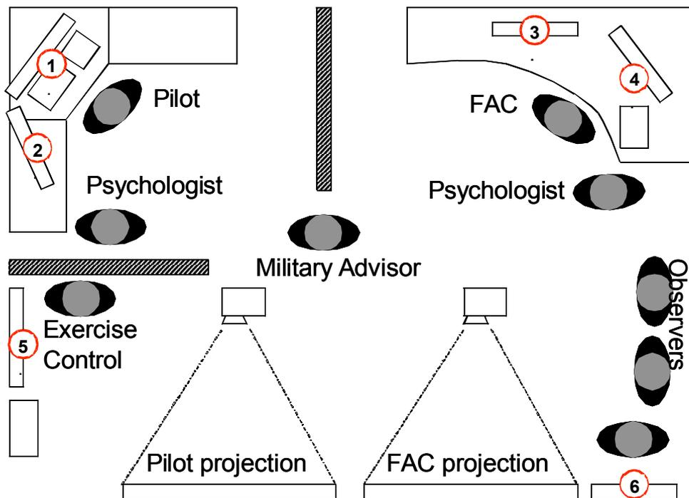
Figure 2: Laboratory Layout for Combat ID MJP
